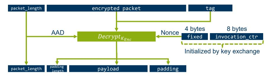
Observation: AES-GCM does not use sequence number but an invocation counter securely initialized through key derivation
